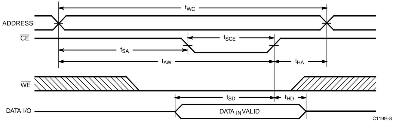
**Write Cycle No. 3 ( $\overline{WE}$  Controlled,  $\overline{OE}$  LOW)<sup>[9, 14]</sup>**
