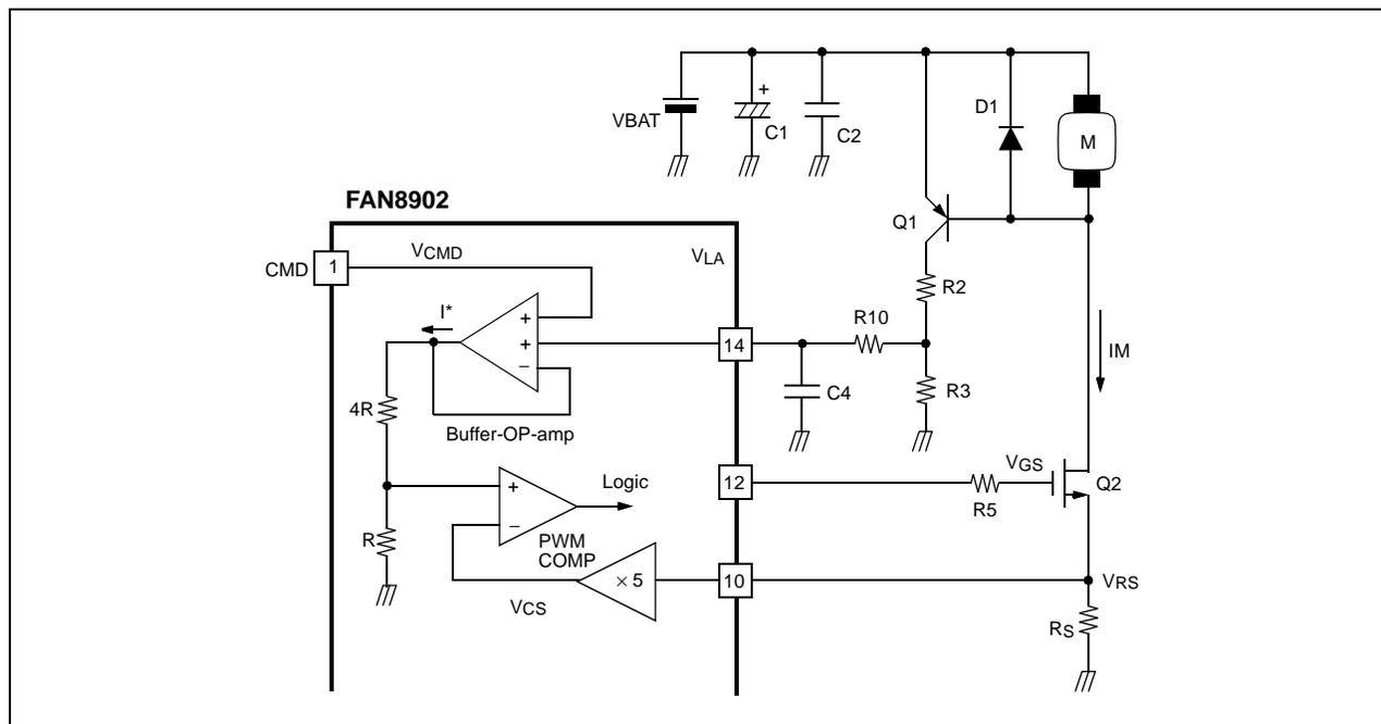
In the steady state, the terminal voltage on a motor is consisted of a back EMF and the voltage drop on the armature resistors. When the motor happens to be stalled, the back EMF becomes zero, and the motor current ( $I_M$ ) is quickly increased until a maximum values.
