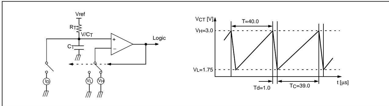
The oscillator timing components can be calculated as follows:
