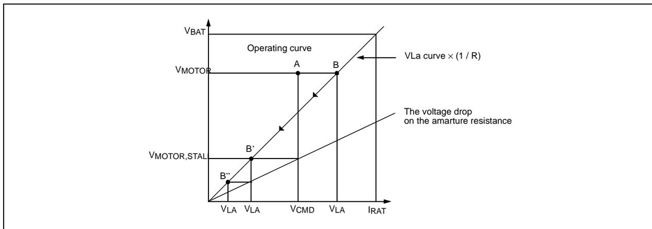
The buffer OP-amp selects the lower command between  $V_{CMD}$  and  $V_{La}$  so as to limit the stalled motor current to very low in the above figure. Because of much larger  $V_{La}$  than  $V_{CMD}$ , the motor operating point stays at A. But the point gradually moves toward B' and then B'' through the curve from the instance of stall as the below figure.
