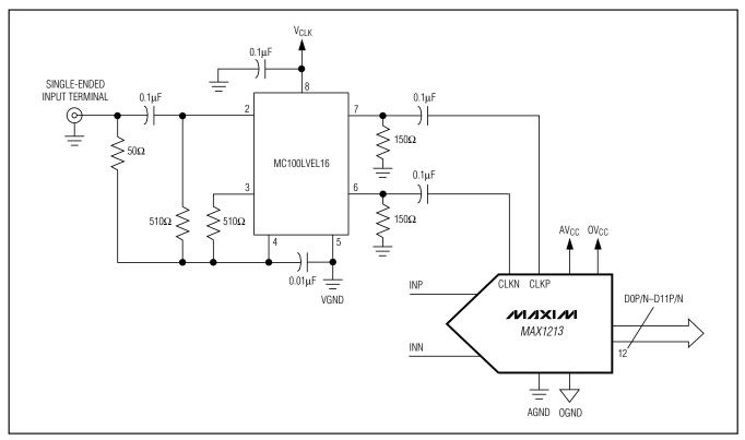
Figure 7. Differential, AC-Coupled, PECL-Compatible Clock Input Configuration
