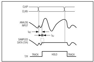
Figure 11. Aperture Jitter/Delay Specifications
