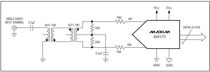
Figure 8. Analog Input Configuration with Back-to-Back Transformers and Secondary-Side Termination
