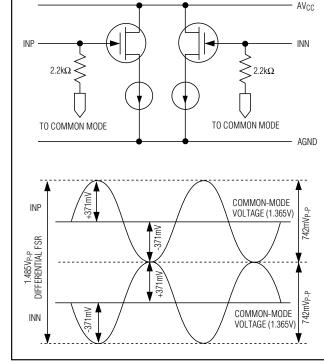
Figure 2. Simplified Analog Input Architecture and Allowable Input Voltage Range
