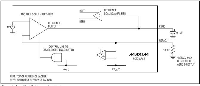
Figure 3. Simplified Reference Architecture
