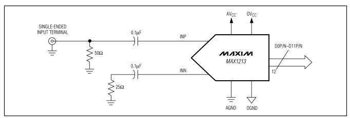
Figure 9. Single-Ended AC-Coupled Analog Input Configuration
