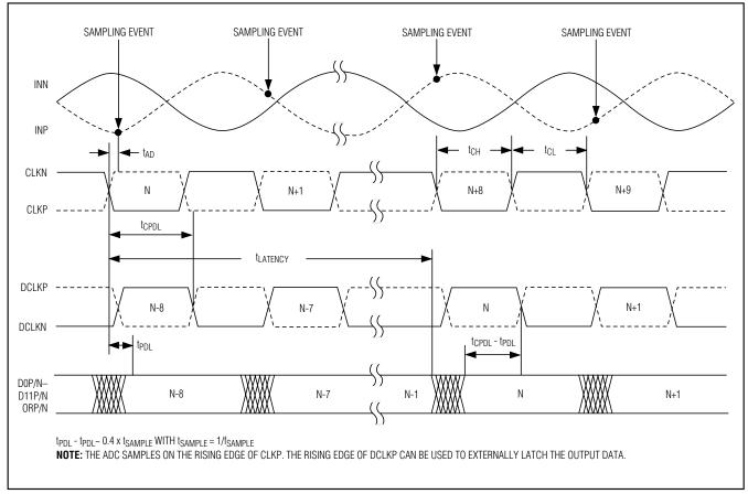
Figure 4. System and Output Timing Diagram
