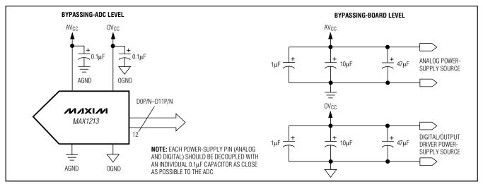
Figure 10. Grounding, Bypassing, and Decoupling Recommendations for MAX1213
