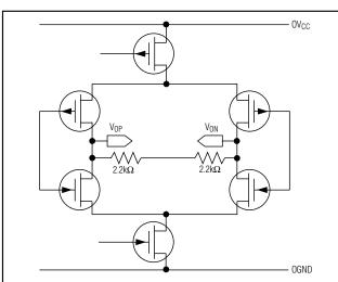
Figure 5. Simplified LVDS Output Architecture
