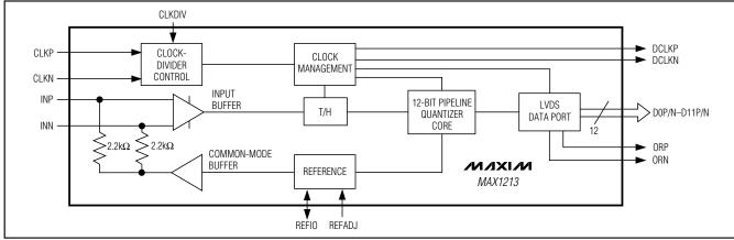
Figure 1. Simplified MAX1213 Block Diagram
