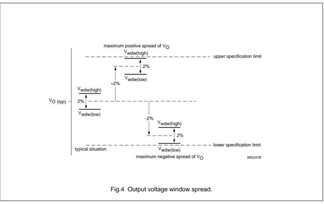
When the output voltage becomes lower than the low limit of the window, a corrective action is taken by a ramp-up of the inductor current during a much longer time. As a result, the DC current level is increased and normal PWM control can continue. The output voltage (including ESR effect) is again within the predefined window.
