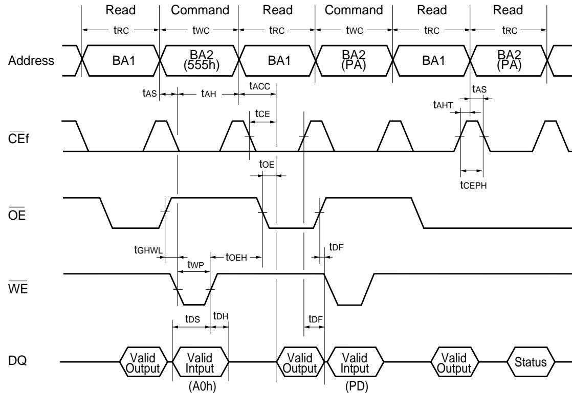
Note : This is example of Read for Bank 1 and Embedded Algorithm (program) for Bank 2.
