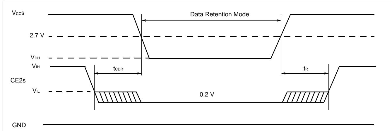
\* : In  $CE2s$  controlled data retention mode, input and input/output pins can be used between -0.3 V to  $V_{CCS} + 0.3 \text{ V}$ .
