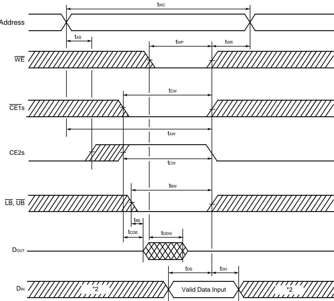
\*1 : If  $\overline{OE}$  is HIGH during the write cycle, the outputs will remain at high impedance.
