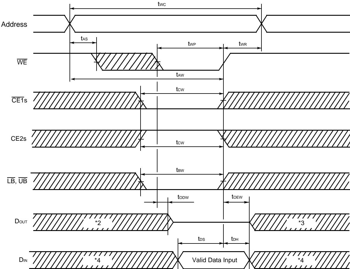
\*1 : If  $\overline{OE}$  is HIGH during the write cycle, the outputs will remain at high impedance.
