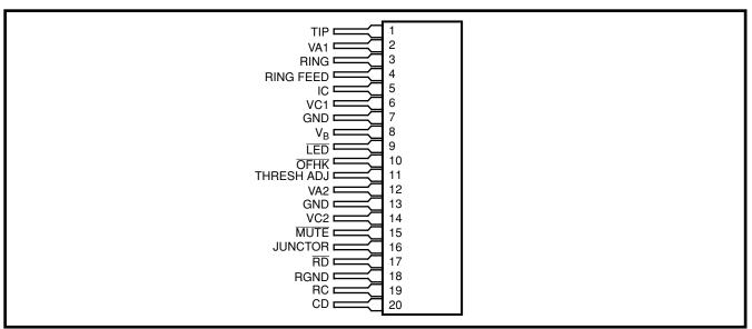
Figure 2 - Pin Connections
