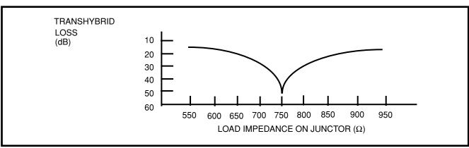
Figure 4 - Return Loss VS Junctor Load Impedance
