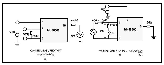
Figure 5 - Transhybrid Loss Test Circuit
