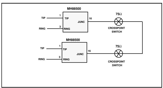
Figure 3 - SLIC Crosspoint Switch Connection
