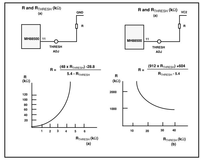
Figure 6 - Off-Hook Threshold Adjust
