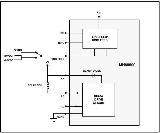
Figure 7 - Relay Drive Circuit
