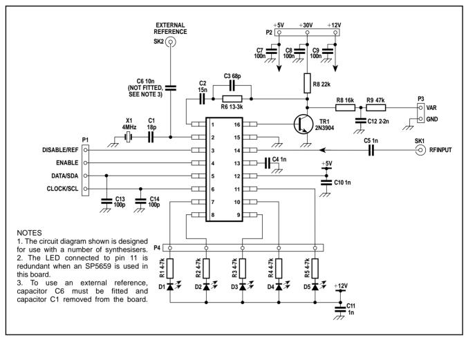
Figure 7 - Test board circuit diagram
