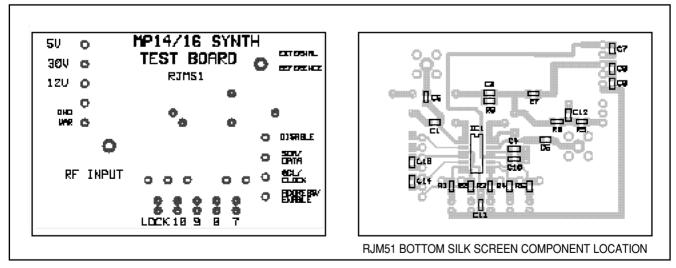
Figure 8 - Test board layout
