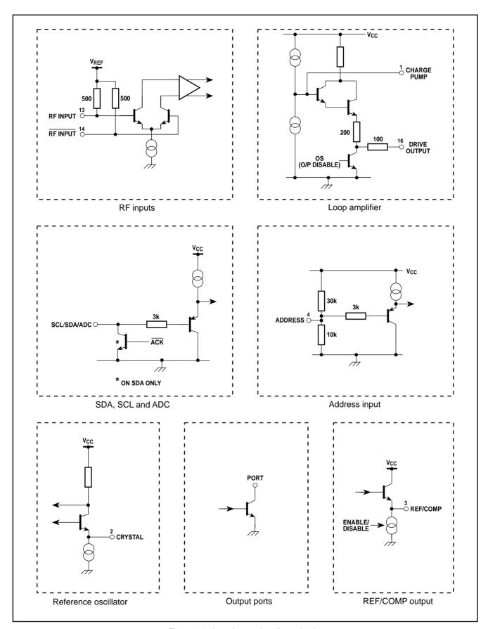
Figure 11 - Input/output interface circuits
