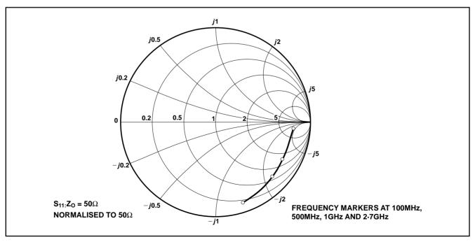
Figure 10 - Typical RF input impedance
