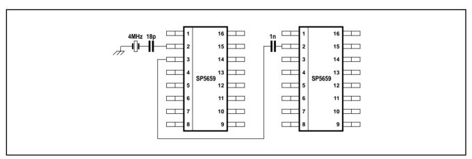
Figure 9 - Two SP5659 devices using a common reference
