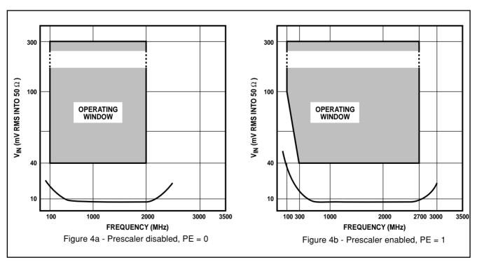
Figure 4 - Typical input sensitivity
