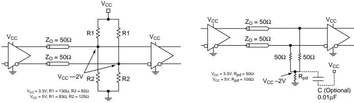
Figure 2a. Parallel Thevenin-Equivalent Termination
