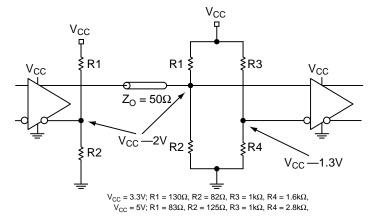
Figure 2c. Terminating Unused I/O
