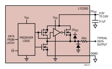
Figure 14. Digital Output Buffer
