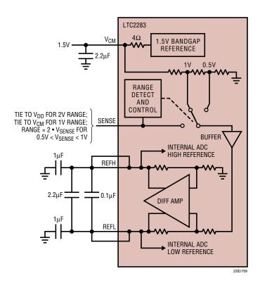
Figure 9. Equivalent Reference Circuit
