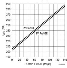
$I_{OVDD}$  vs Sample Rate, 5MHz Sine Wave Input, -1dB,  $OV_{DD}$  = 1.8V
