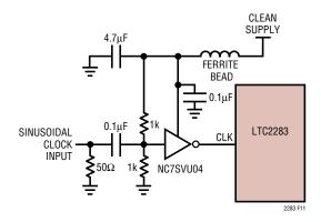
Figure 11. Sinusoidal Single-Ended CLK Drive
