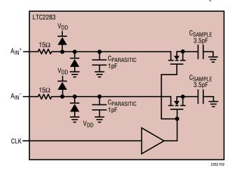
Figure 2. Equivalent Input Circuit
