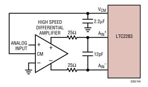
Figure 4. Differential Drive with an Amplifier
