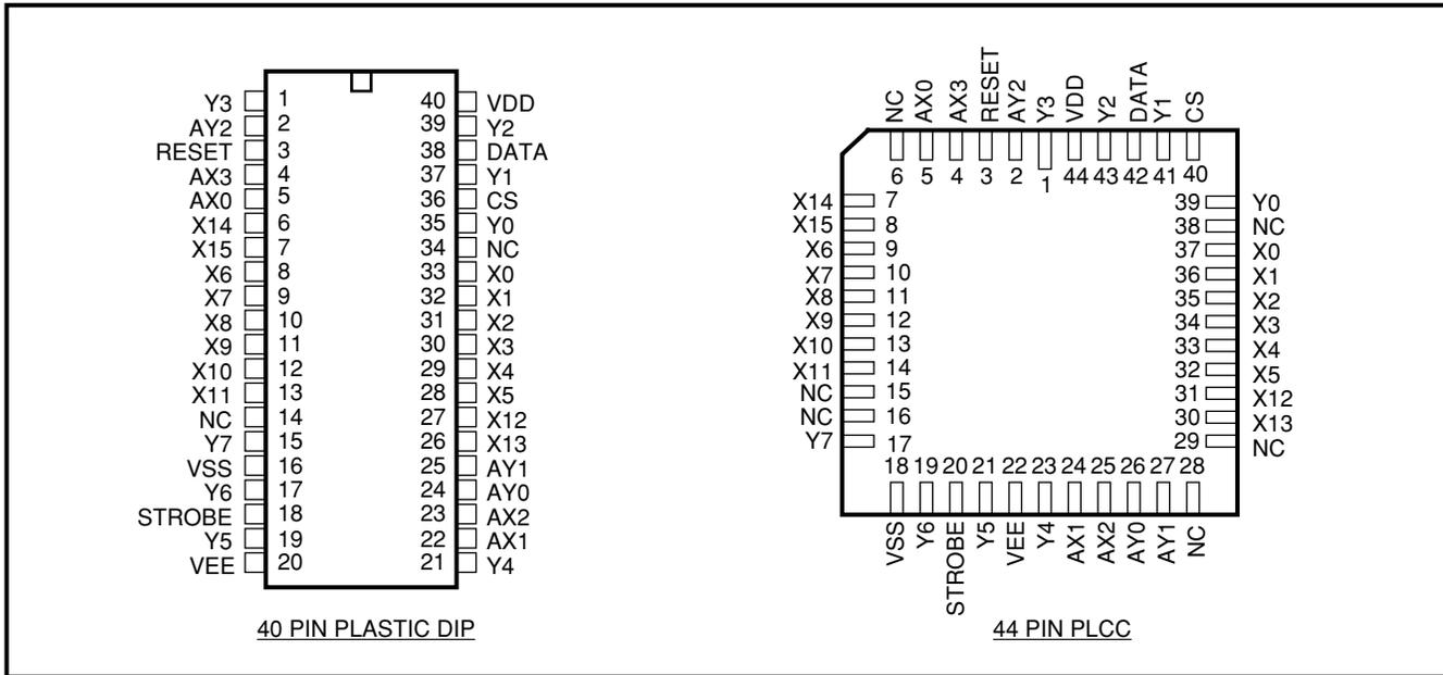
Figure 2 - Pin Connections
