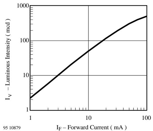
Figure 6 Luminous Intensity vs. Forward Current
