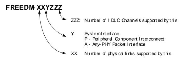
There are 4 product variants in the second generation FREEDM product family. These product variants are specifically designed to address the unique requirements of different networking equipment. For example, the dial-access equipment terminates a large number of communication sessions with remote users. A fully channelized DS3
