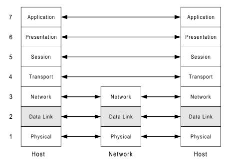
Many protocol choices are frequently available for each layer, and some overlap in functionality with several layers. On data link layer, the High Level Data Link Control (HDLC) specification is one of the most popular protocol used to encapsulate upper layer protocols, such as TCP/IP, for transmission over the wide area network.
