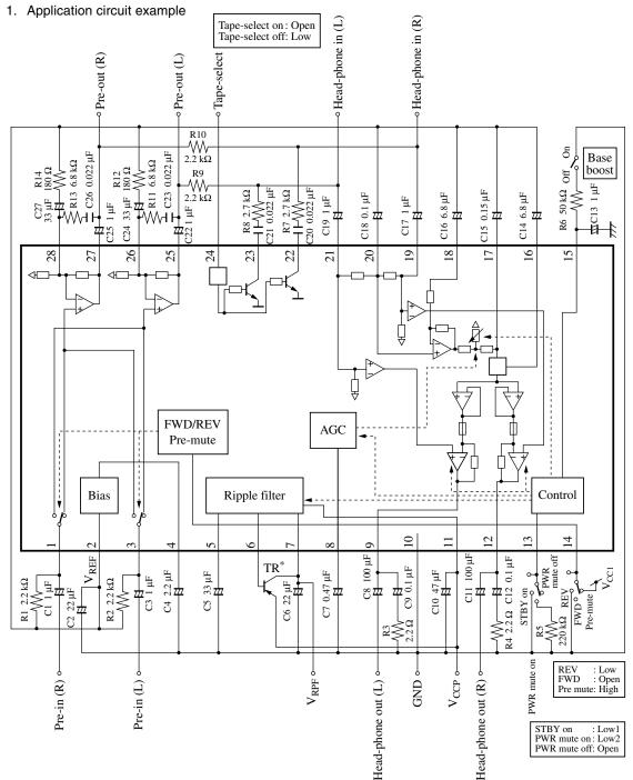
Note) \*: The low V<sub>CE(SAT)</sub> PNP TR be used as TR.
