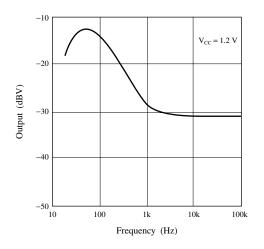
Distortion and amplitude characteristics of headphone amp.
