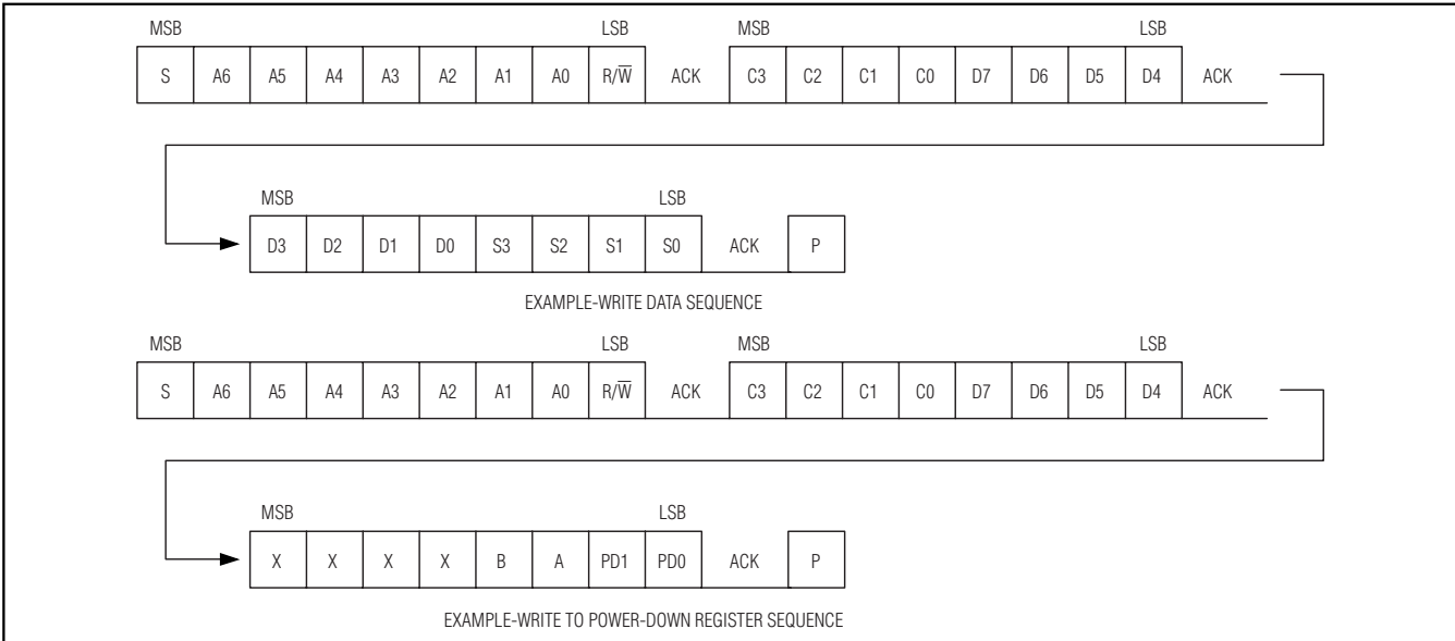
Figure 6. Example-Write Command Sequences
