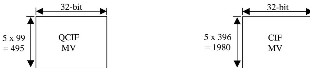
Figure 24-5. Motion Vector Configuration for QCIF/CIF Image
