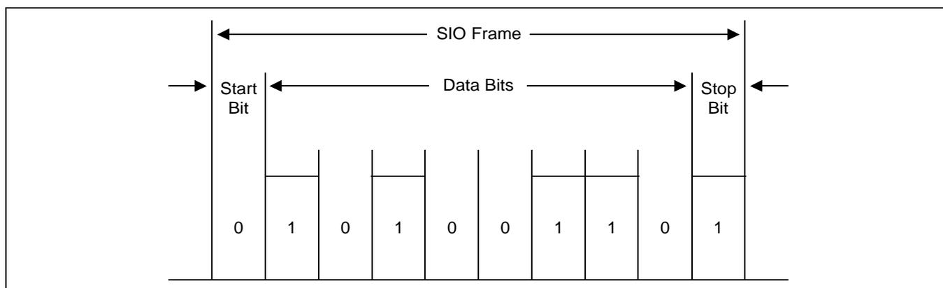
Figure 11-4. Serial I/O Frame Timing Diagram (Normal UART)
