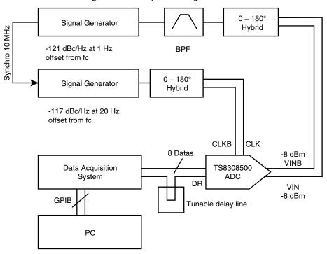
Figure 15. Single-ended Analog and Clock Input Configuration
