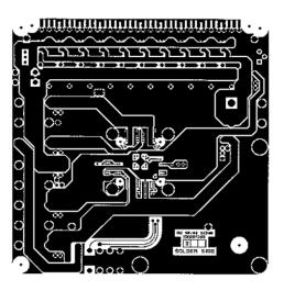
**Figure 13.** TSEV8308500GL Evaluation Board: Components Placement
