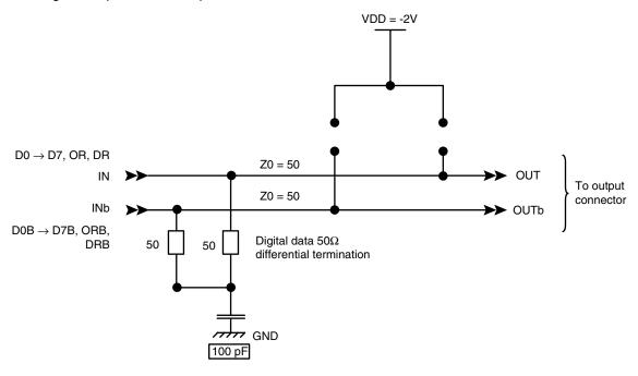
Figure 9. Board Digital Outputs Option Using MC100EL16 Differential Receivers
