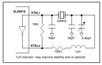
Figure 31 - Crystal Oscillator Circuit
