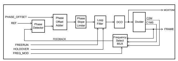
Figure 28 - Block Diagram of the PLL Module
