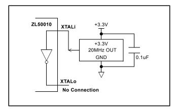
Figure 32 - External Clock Oscillator Circuit
