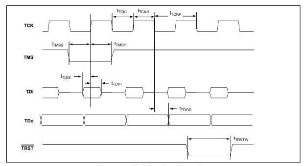
Figure 49 - JTAG Test Port Timing Diagram
