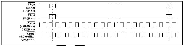
Figure 8 -  $\overline{FPo0}$  and  $\overline{CKo0}$  Output Timing when the CKFP0 bit = 0
