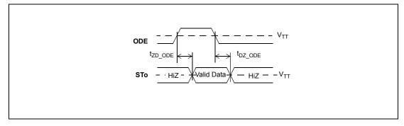
Figure 47 - Output Driver Enable (ODE)
