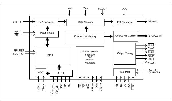
Figure 1 - ZL50010 Functional Block Diagram
