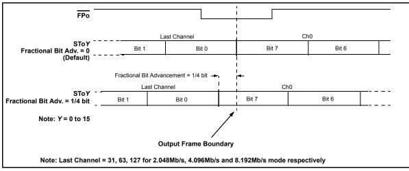
Figure 19 - Fractional Output Bit Advancement Timing Diagram
