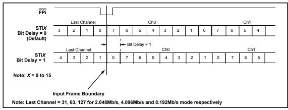
Figure 16 - Input Bit Delay Timing Diagram
