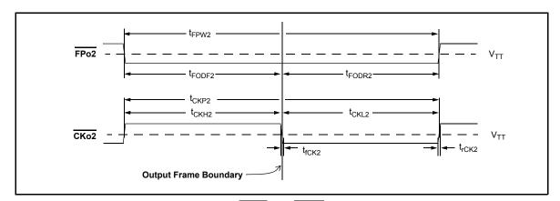
Figure 43 - FPo2 and CKo2 Timing Diagram
