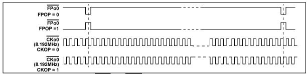
Figure 9 -  $\overline{FP00}$  and  $\overline{CK00}$  Output Timing when the CKFP0 bit = 1
