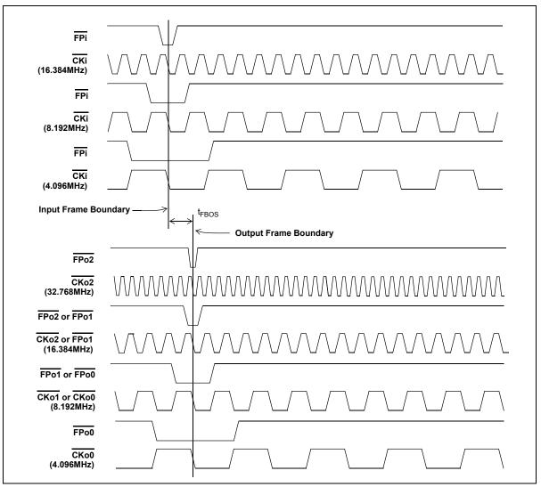
Figure 40 - Input and Output Frame Boundary Offset
