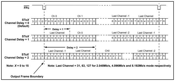
Figure 17 - Output Channel Delay Timing Diagram
