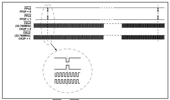
Figure 12 -  $\overline{FPo2}$  and  $\overline{CKo2}$  Output Timing when the CKFP2 bit = 0
