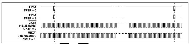
Figure 10 - FPo1 and CKo1 Output Timing when the CKFP1 bit = 0
