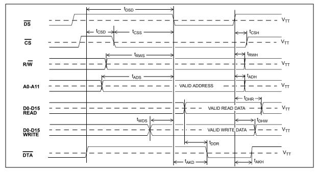
Figure 48 - Motorola Non-Multiplexed Bus Timing
