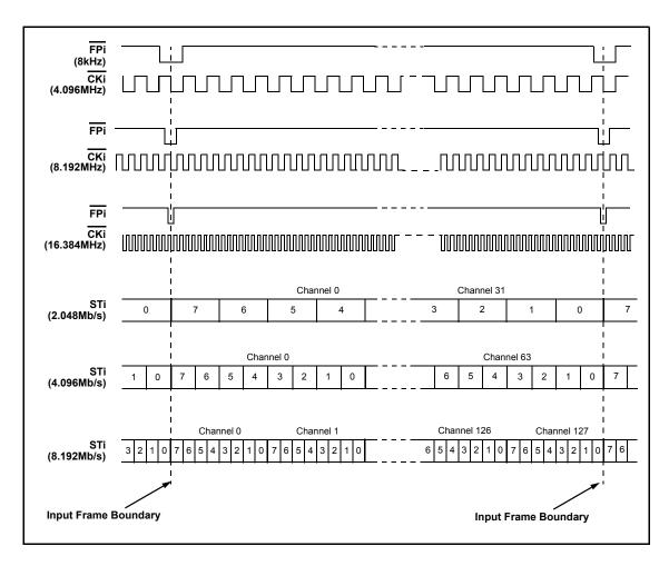
Figure 7 - ST-BUS Input Timing for Various Input Data Rates
