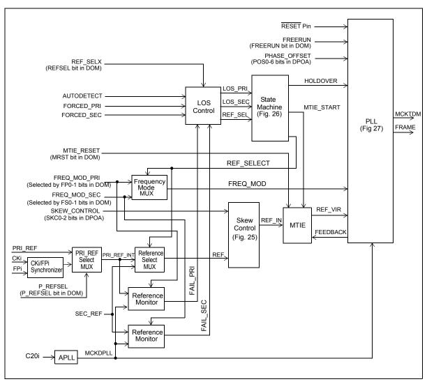
Figure 25 - DPLL Functional Block Diagram
