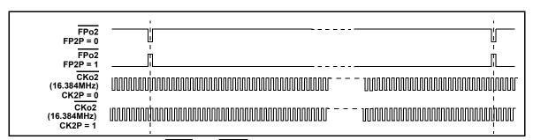
Figure 13 - FPo2 and CKo2 Output Timing when the CKFP2 bit = 1
