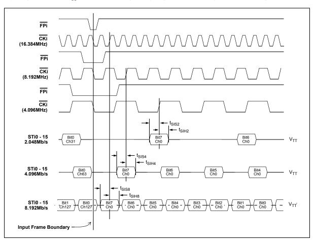
Figure 44 - ST-BUS Inputs (STi0 - 15) Timing Diagram
