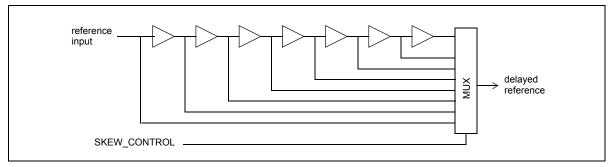
Figure 26 - Skew Control Circuit Diagram
