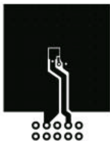
a) 56°C/W when mounted on a 1 in 2 pad of 2 oz copper
