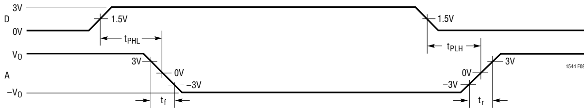
Figure 8. V.10, V.28 Driver Propagation Delays
