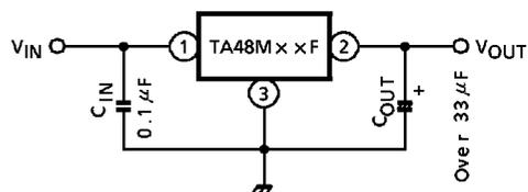
Connect the input terminal and GND, and the output terminal and GND, by capacitor respectively. The capacitances should be determined experimentally. In particular, adequate investigation should be made so that there is no problem even at time of high or low temperature.
