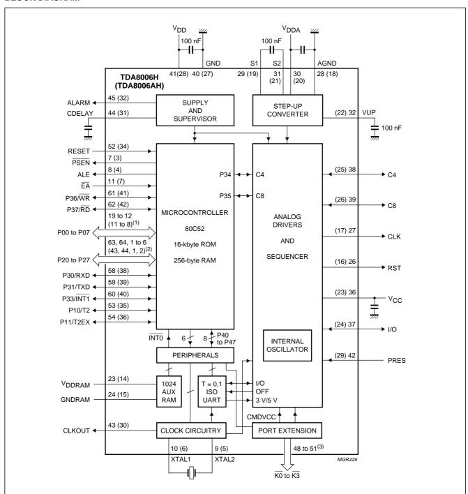
Minimum value for capacitor between  $V_{\text{DDA}}$  and AGND is 2.2  $\mu\text{F}.$
