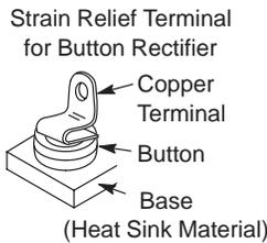
The base heat sink may be of various materials whose shape and size are a function of the individual application and the heat transfer requirements.
