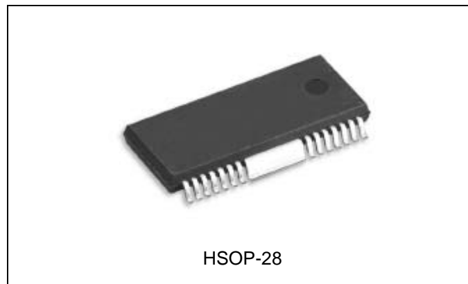
Figure 1. Package Type of AM5665
