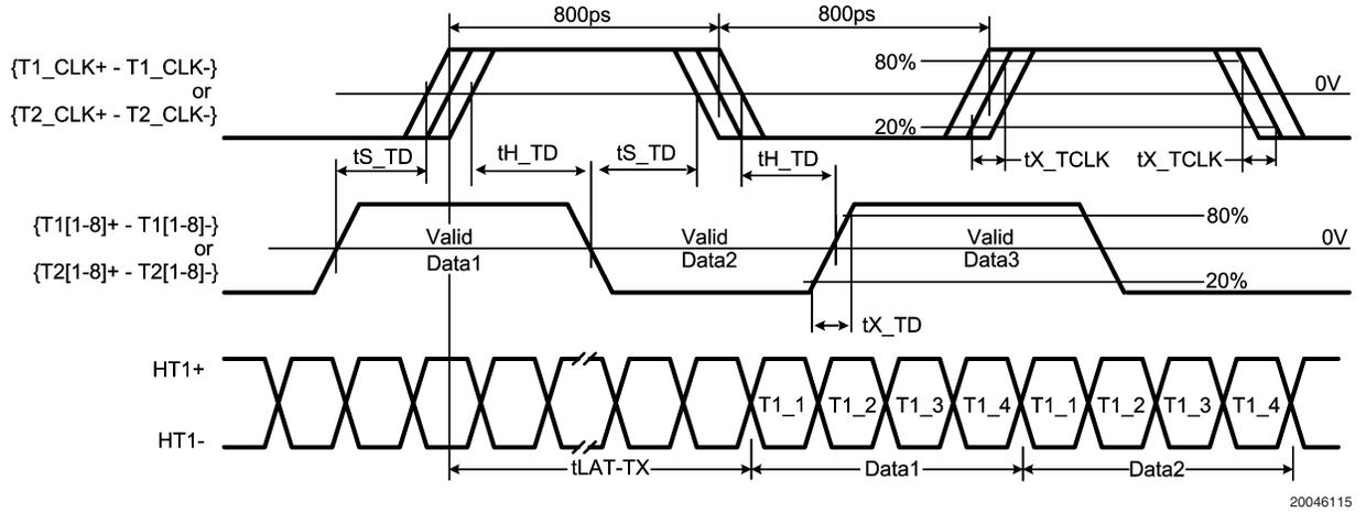
FIGURE 9. Transmit Data Timing
