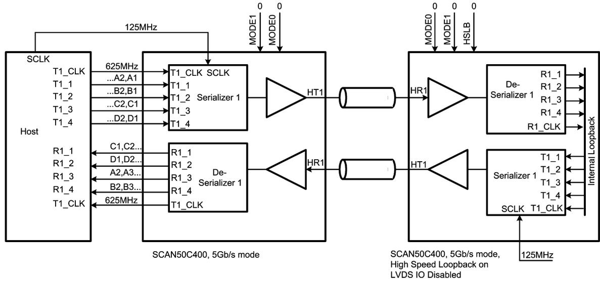
FIGURE 7. SCAN50C400 in High-Speed Loopback (5 Gbps Shown)
