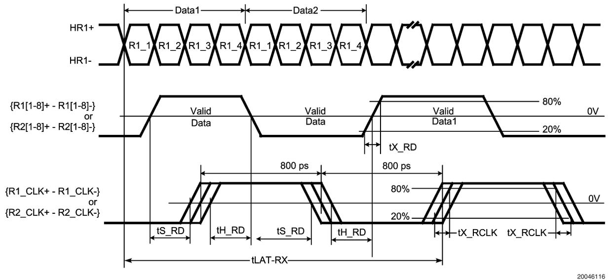
FIGURE 10. Receive Data Timing
