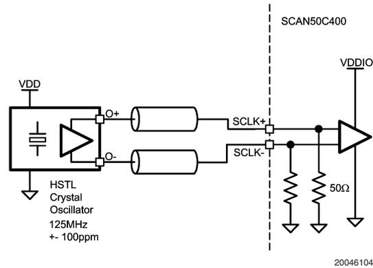
FIGURE 1. SCLK± Driven by HSTL Clock Driver / Crystals
