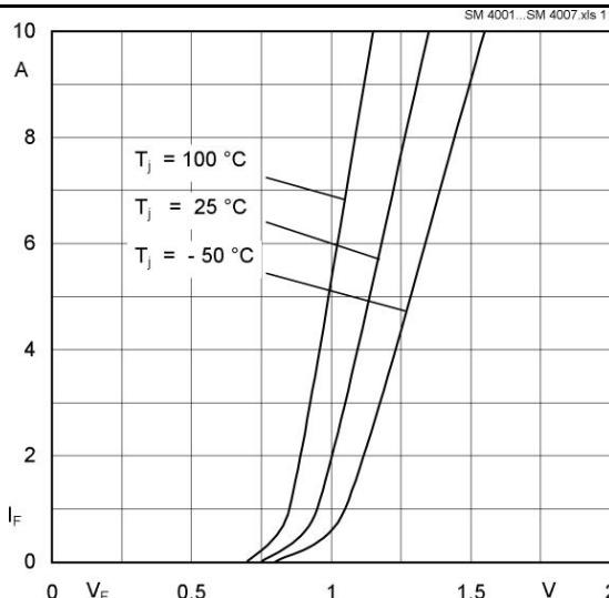
Fig. 1 Forward characteristics ( typical values )
