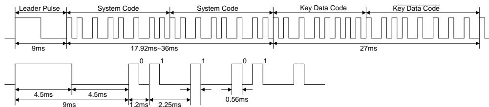
Continuous Transmission Waveform
