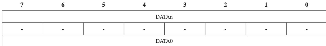
DATA0 is the first received (or transmitted) byte, DATAn is the last one.
