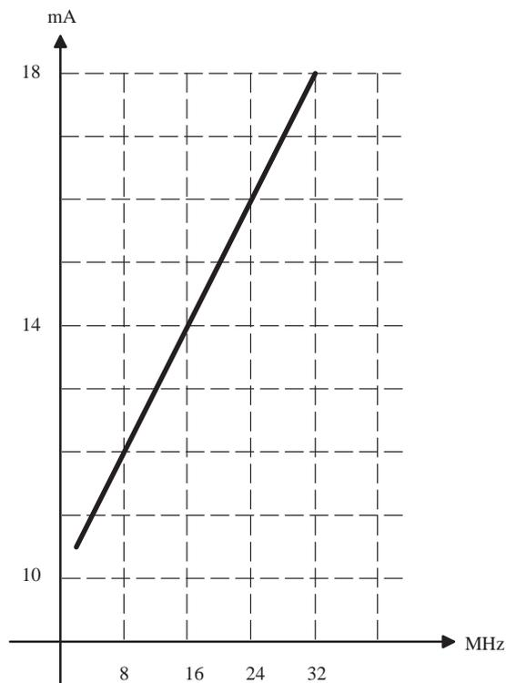
Figure 33.  $I_{CC}$  Versus Clock Frequency
