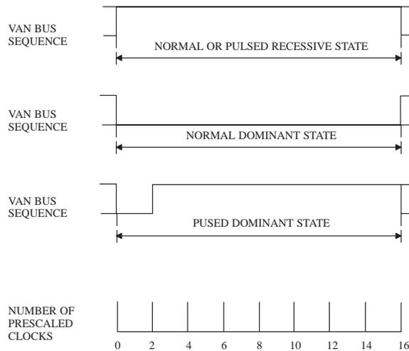
**Figure 7. State Encoding.**
