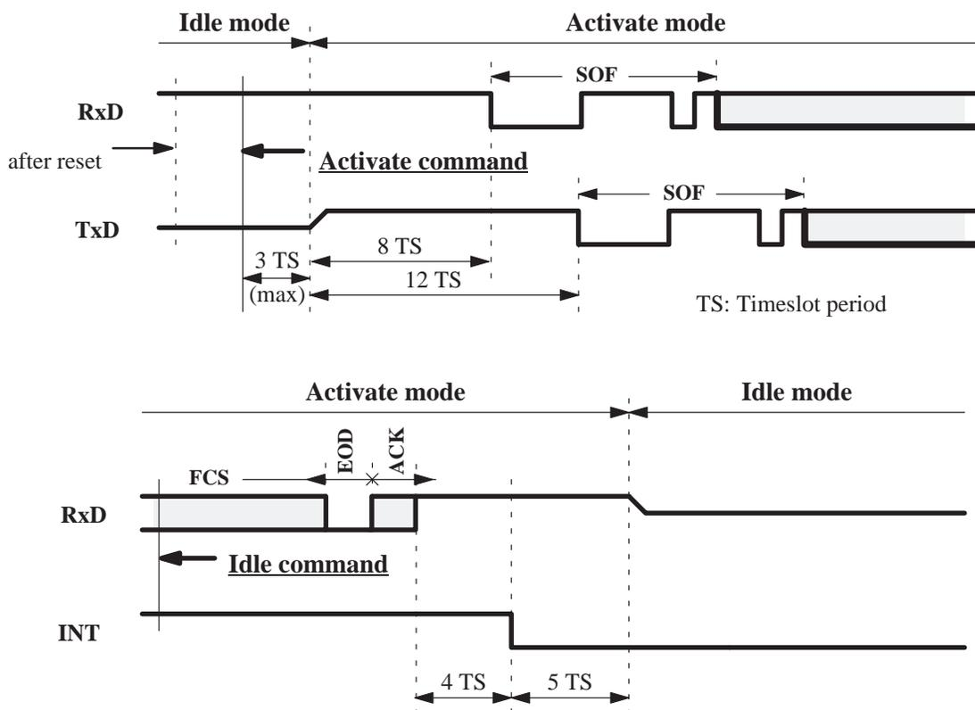
Figure 30. Idle and activate timings
