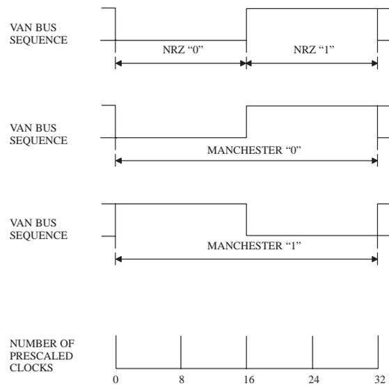
**Figure 11. Data Encoding.**
