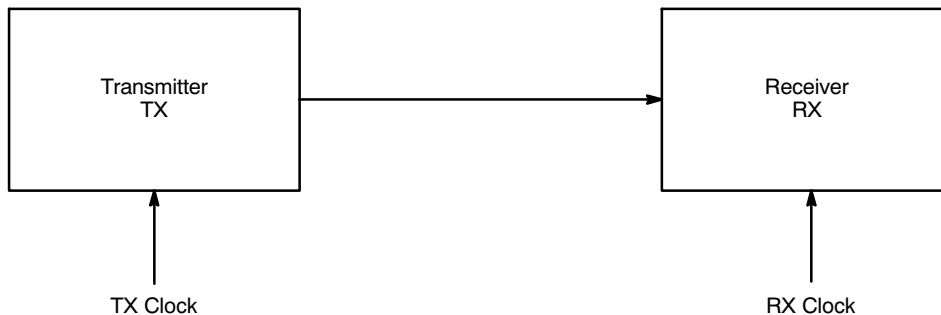
Figure 33. Example of a Serial Data Transmission System
