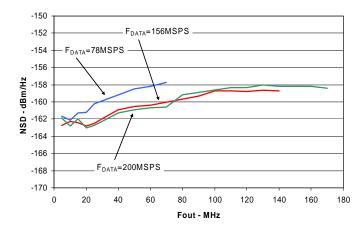
Figure 17. Noise Spectral Density vs. Fout, 2x Interpolation
