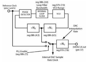
Figure 32. Internal Clock Architecture of AD9779
