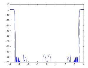
Figure 40. Interpolation/Modulation Combination of -4f<sub>DAC</sub>/8 Filter in Odd Mode
