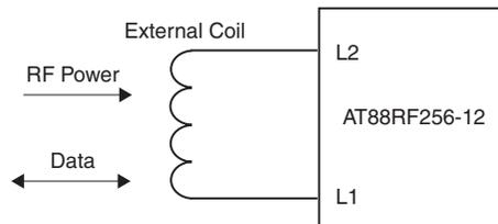
Typical Coil Inductance @125 kHz is ~10.1 mH
