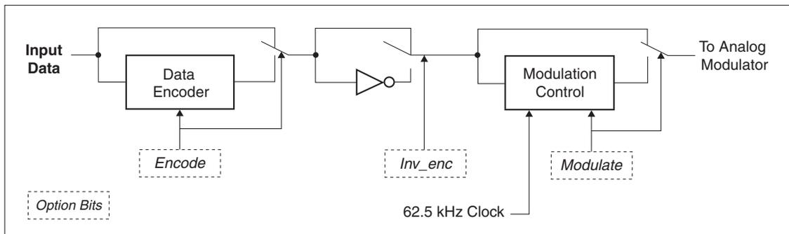
**Data Transmission Protocol (Bit rate equals 16 clocks per bit)**
