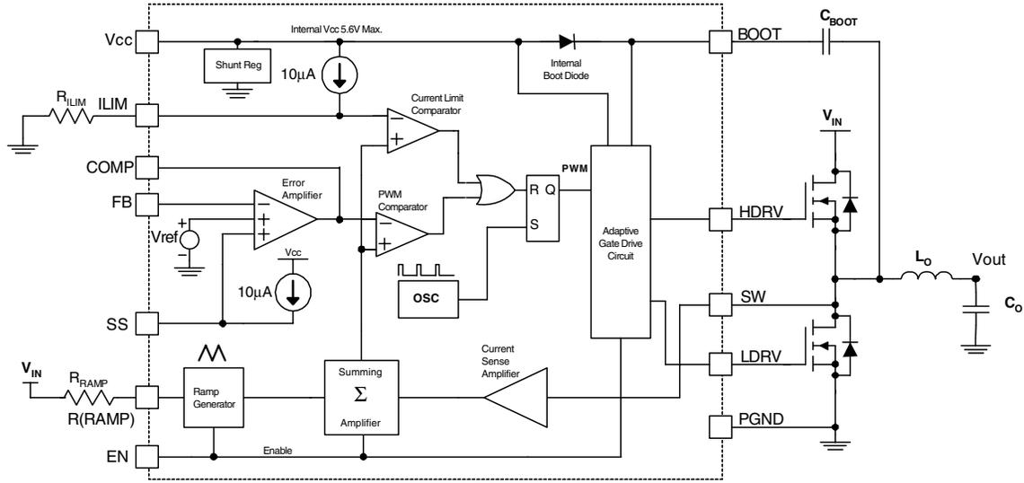
Figure 20. Block Diagram
