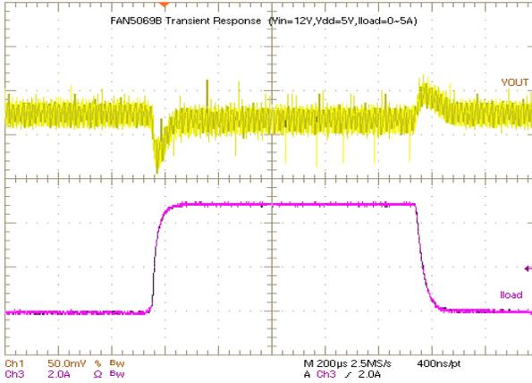
Figure 4. PWM Load Transient (0 to 5A)
