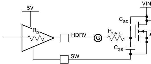
Figure 23. Drive Equivalent Circuit
