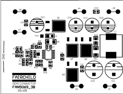
Figure 26. Assembly Diagram
