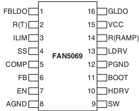
**Figure 2. Pin Assignment**
