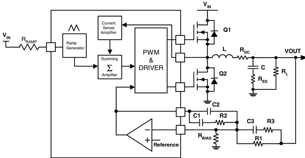
**Figure 24. Closed Loop System with Type 3 Network**
