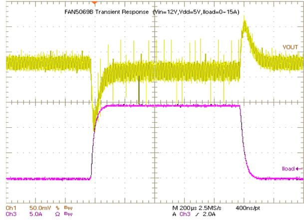
Figure 6. PWM Load Transient (0 to 15A)
