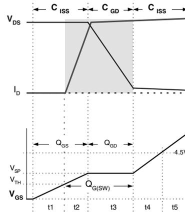
Figure 22. Switching Losses and  $Q_G$
