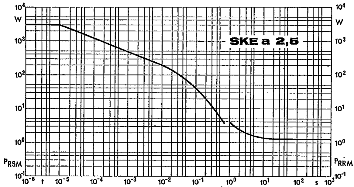
Fig. 11 c Rated reverse power dissipation vs. time
