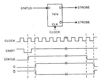
If continuously converting, the STATUS (E.O.C.) output can be NORed with the converter clock, as shown below, to produce a positive strobe pulse 1/2 period wide, 1/2 period after the STATUS output has gone low. The rising edge of this pulse can be used to latch data after each conversion.
