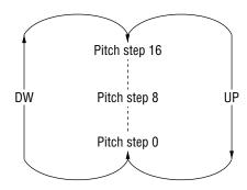
MSM6722 ····· The pitch step does not change if a signal is input to the UP • C (DW • C) pin when the pitch step is 16 or 0.
