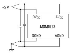
Do not supply the power to the analog section and the logic section from separate power sources; otherwise latch-up may occur.
