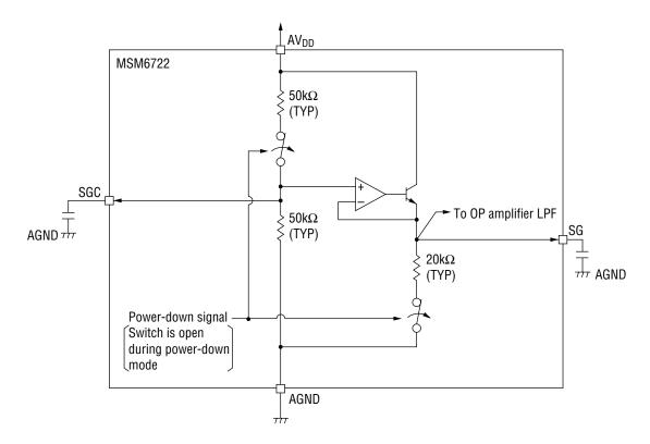
The SG signal is reference voltage (signal ground) for internal OP amplifiers and LPF. Install a capacitor between the SGC pin and AGND and between the SG pin and AGND respectively in order to make the SG signal noiseless. It is recommended to install an approx.  $1\mu$  capacitor, which should be determined after evaluating the tone quality.
