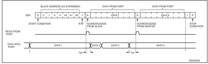
Figure 10. I/O READ mode (input)
