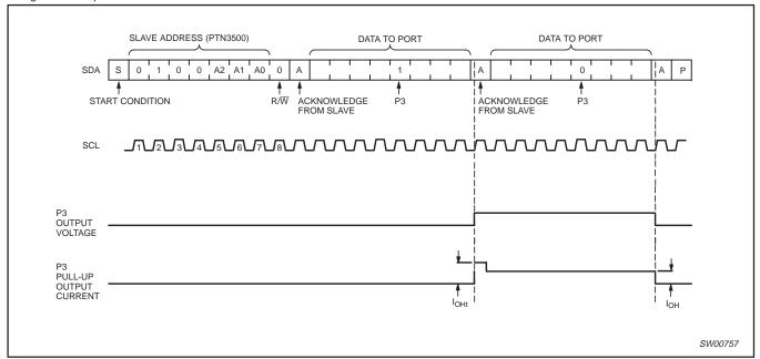
Figure 11. Transient pull-up current  $I_{\text{OHt}}$  while P3 changes from LOW-to-HIGH and back to LOW
