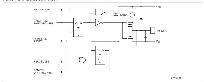
Figure 7. Simplified schematic diagram of each I/O
