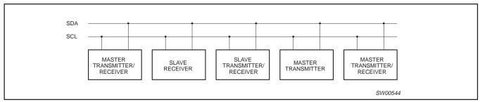
Figure 5. System configuration
