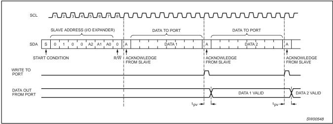
Figure 9. I/O WRITE mode (output)
