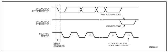
Figure 6. Acknowledgment on the I<sup>2</sup>C-bus
