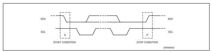
Figure 4. Definition of start and stop conditions
