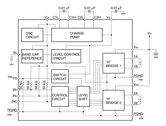
**Note** The power-saving mode is set when the PS pin goes high. In this mode, the voltage of the charge pump circuit is lowered and the ON resistance of the H bridge driver transistor increases, limiting the current.
