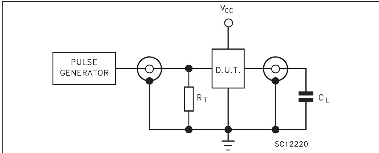
$C_L = 15/50\text{pF}$  or equivalent (includes jig and probe capacitance)
