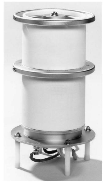
In addition to 300 W of heater power, the tube dissipates from 100 W per ampere average anode current, rising to 300 W/A at the highest rates of rise and fall of anode current.
