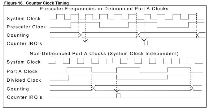
The two remaining clock sources are coming from the PA[0] or PA[3] terminals. Refer to the Figure 12 on page 14 for details. Both sources can be either debounced (Ck[11] or Ck[8]) or direct inputs, the input polarity can also be chosen. The output after the debouncer polarity selector is named PA3, PA0 respectively. For the debouncer and input polarity selection refer to chapter 7.2.4.
