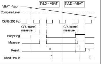
power supply voltage was greater than the detection level value. If read 1, the power supply voltage was lower than the detection level value. During each read while **Busy=1** the **VidResult** is not guaranteed. The interrupt request can be masked (default) (**MaskIRQVLD** bit).
