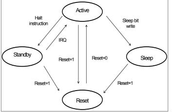
sleep mode only the voltage regulator and the reset input are active. The RAM data integrity is maintained. Sleep mode may be canceled only by a high level of min 10µs at the Reset terminal or by the selected port A input reset combination, if option **InpResSleep** in register **OPTFSelPB** is turned on.
