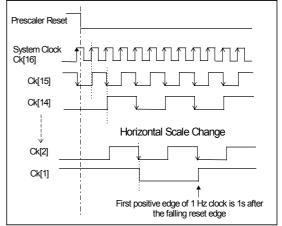
With DebSel = 1 one may choose either the Ck[11] or Ck[14] debouncer frequency by selecting the corresponding metal mask option (*ROM Version only*). Relative to 32kHz the corresponding max. debouncer times are then 2 ms or 0.25 ms. For the metal mask selection refer to chapter 19.1.4.
