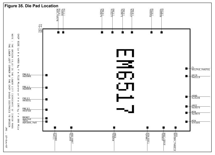
The Pad Test is twice on the circuit, it can be bound either on top or on the left side. Internally the two pads test are connected together by a metal wire.
