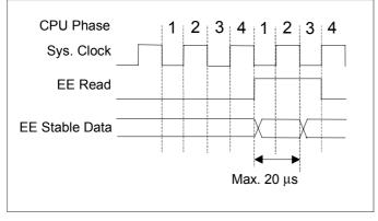
EEPROM access time is max. 20µs : Data is available in RegEEPDataL and RegEEPDataH registers at the instruction following the read access on 32kHz system clock The read signal is 1.5 system clock wide. The CPU reads at end of phase 3.
