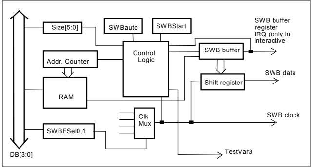
Figure 22. Serial Write Buffer Architecture
