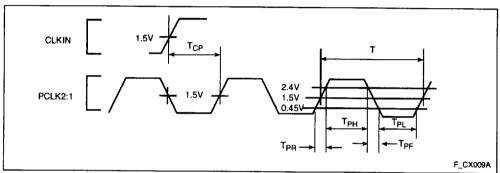
Figure 8. Input and Output Clocks Waveform
