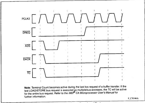
Figure 45. Terminal Count Functional Timing
