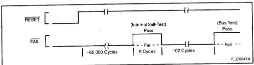
Figure 46. FAIL Functional Timing
