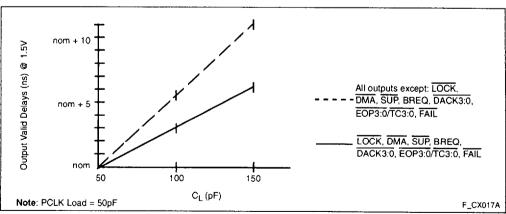
Figure 16. Output Delay or Hold vs. Load Capacitance
