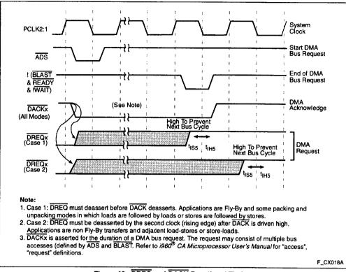
Figure 43. DREQ and DACK Functional Timing
