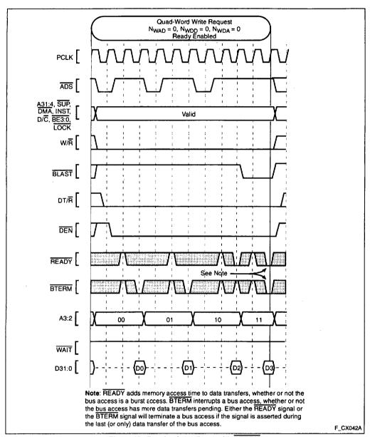
Figure 40. Terminating a Burst with BTERM
