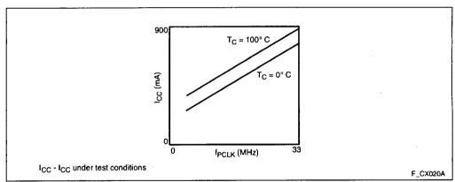
Figure 18. I<sub>CC</sub> vs. Frequency and Temperature
