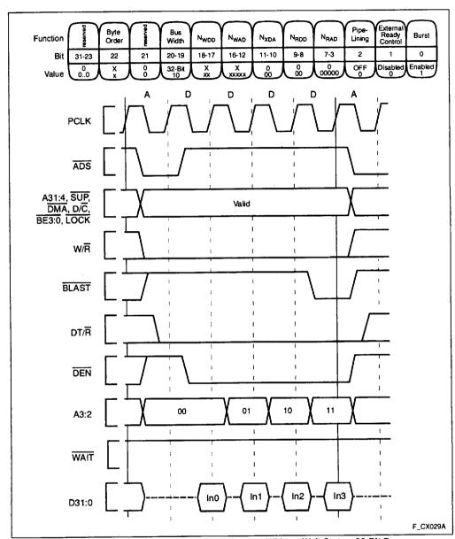
Figure 27. Burst, Non-Pipelined Read Request Without Walt States, 32-Bit Bus
