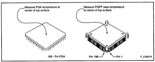
Figure 5. Measuring 80960CA PGA and PQFP Case Temperature
