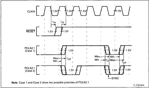
Figure 22. Clock Synchronization in the 2-x Clock Mode
