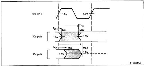
Figure 10. Output Delay and Float Waveform
