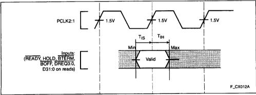
Figure 11. Input Setup and Hold Waveform
