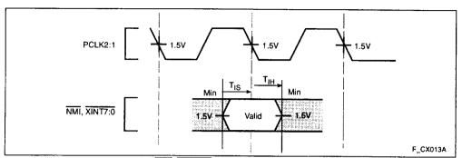
Figure 12. NMI, XINT7:0 Input Setup and Hold Waveform
