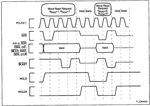
Figure 42. HOLD Functional Timing
