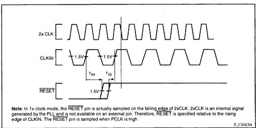
Figure 23. Clock Synchronization in the 1-x Clock Mode
