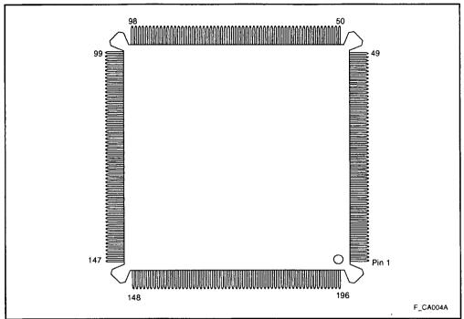
Figure 4. 80960CA PQFP Pinout (View from Top Side)
