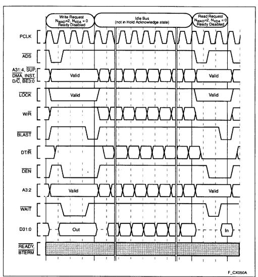
Figure 49. Idle Bus Operation
