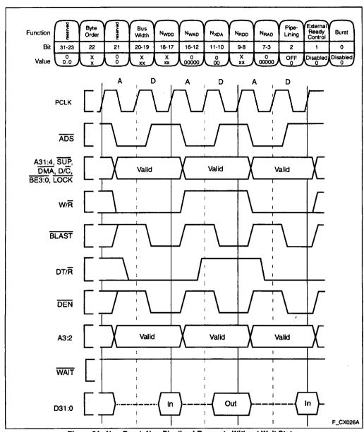
Figure 24. Non-Burst, Non-Pipelined Requests Without Wait States
