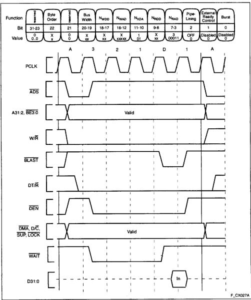
Figure 25. Non-Burst, Non-Pipelined Read Request With Wait States
