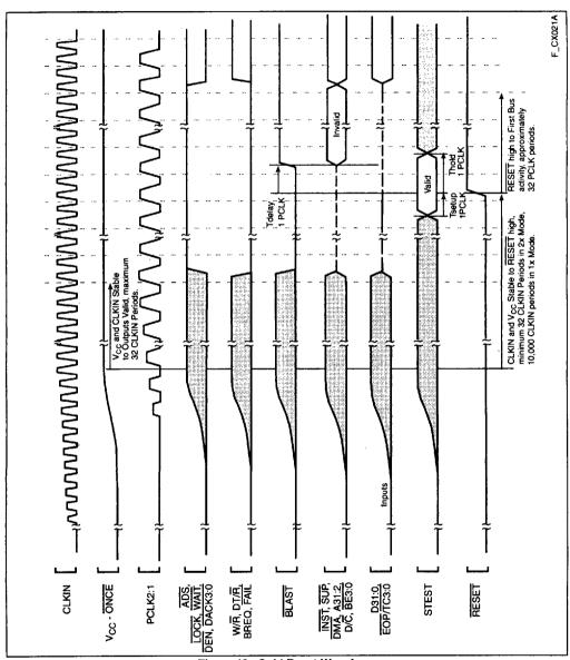
Figure 19. Cold Reset Waveform
