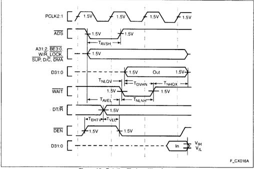
Figure 15. Relative Timings Waveforms
