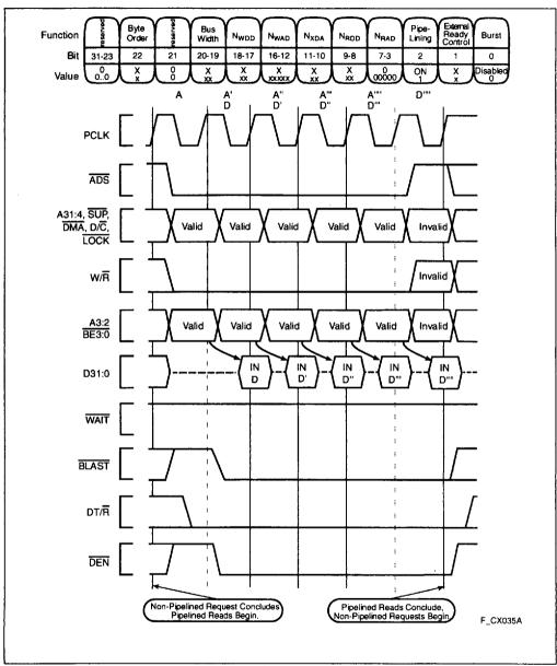
Figure 33. Non-Burst, Pipelined Read Request Without Wait States, 32-Bit Bus
