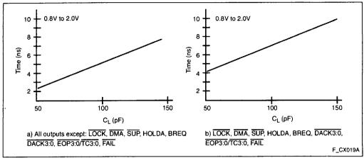
Figure 17. Rise and Fall Time Derating at Highest Operating Temperature and Minimum V<sub>CC</sub>
