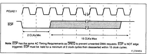
Figure 44. EOP Functional Timing
