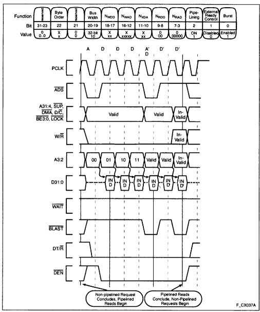
Figure 35. Burst, Pipelined Read Request Without Wait States, 32-Bit Bus
