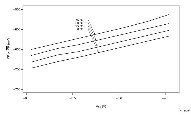
Figure 8. Typical MK or  $\overline{MK}$  vs. Vss for IMOD = 40 mA
