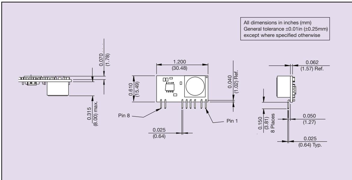
Figure 2: Mechanical Drawing - Vertical Mount Version
