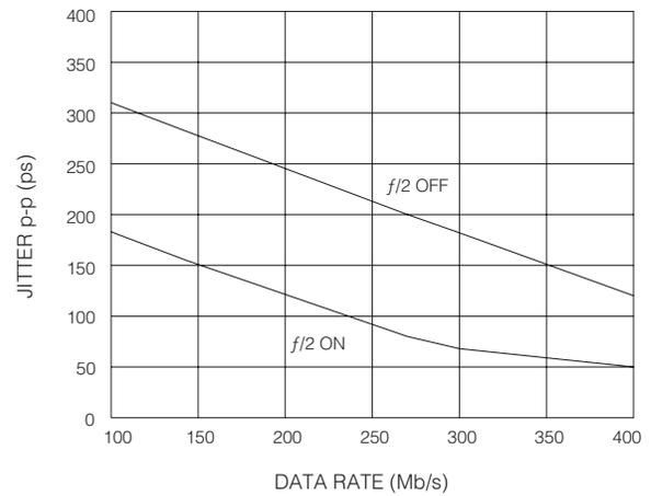
Fig. 12 Output Jitter
