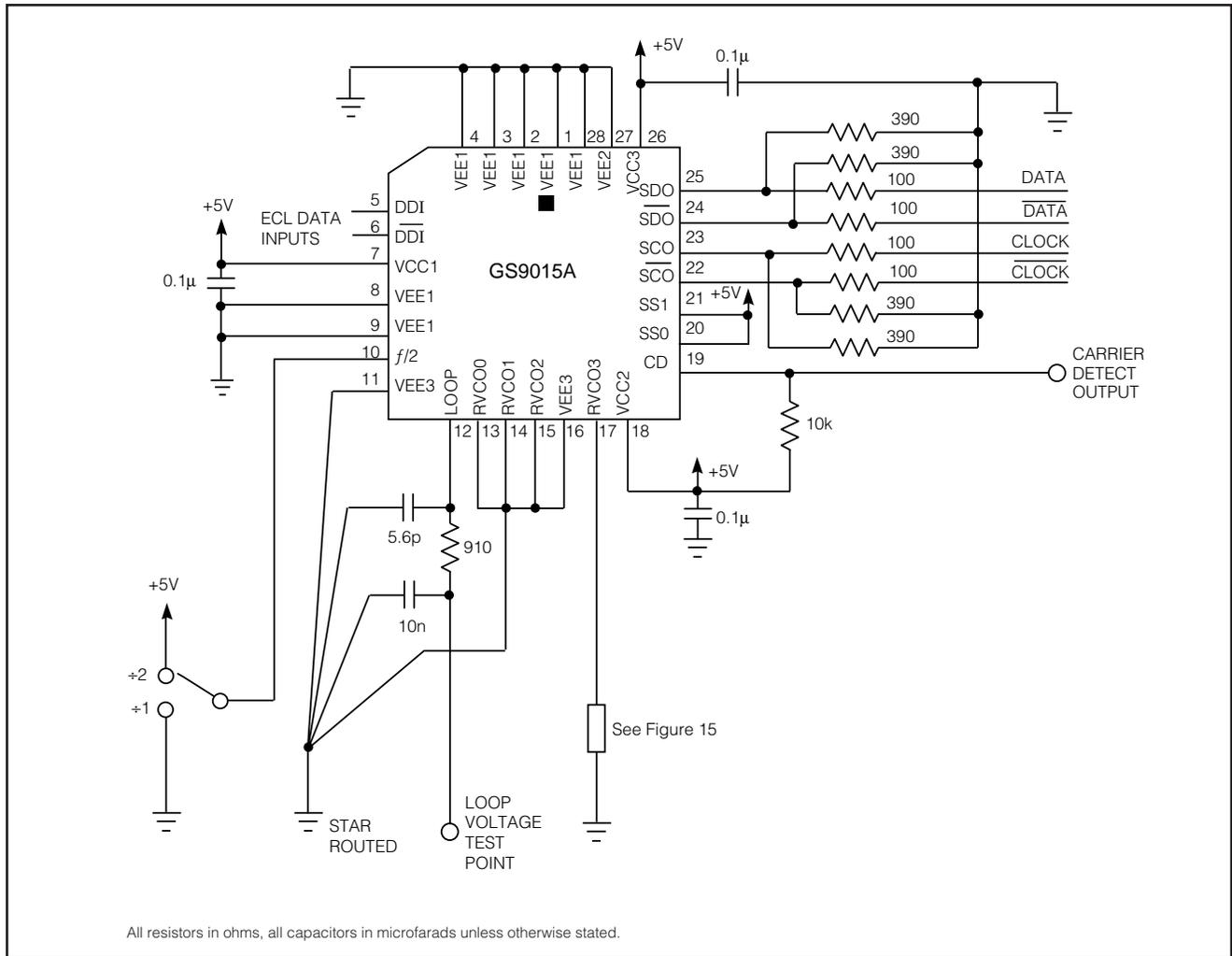
Fig. 13 GS9015A Typical Test Circuit Using +5V Supply
