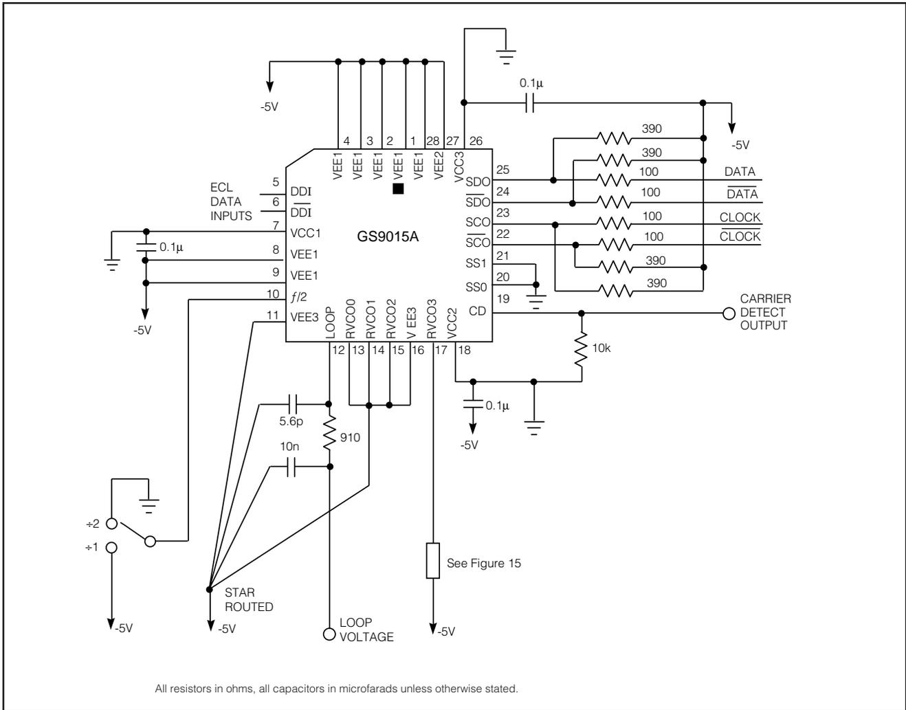
Fig. 14 GS9015A Typical Test Circuit Using -5V Supply
