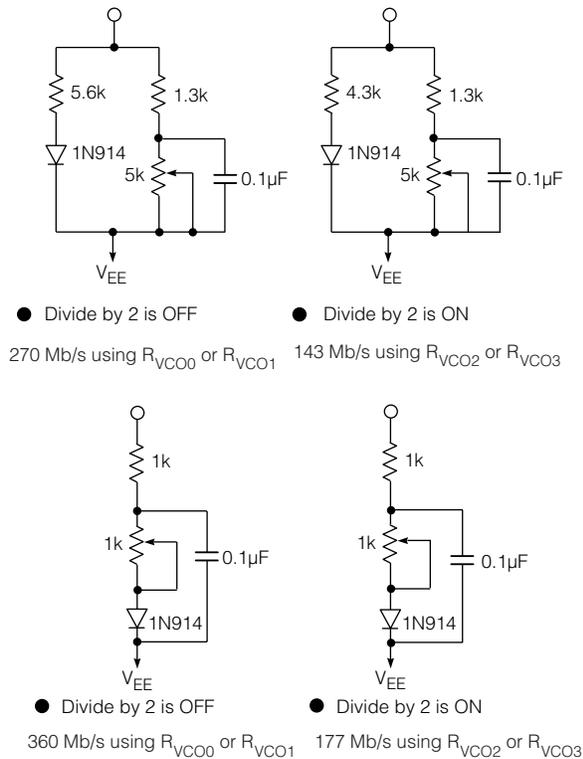
Fig. 15 Frequency Setting Resistor Values
