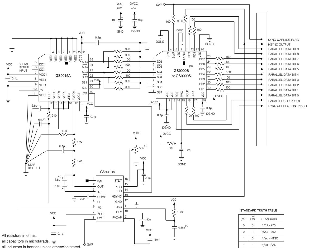
(1) To reduce board space, the two anti-series 6.8  $\mu$ F capacitors (connected across pins 2 and 3 of the GS9010A) may be replaced with a 1.0  $\mu$ F non-polarized capacitor provided that:
