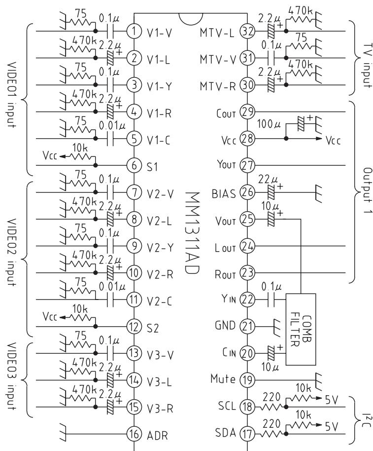
Notes 1 : V<sub>OUT</sub> is set at 4.4V and C<sub>IN</sub> at 4.3V.
