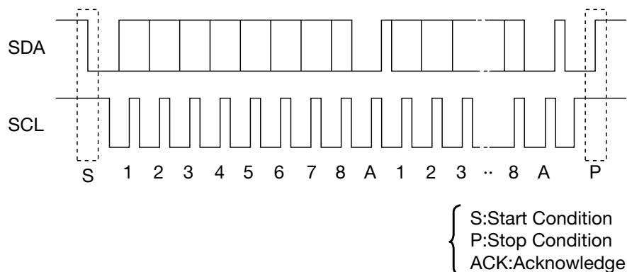
The I<sup>2</sup>C BUS is a BUS system developed by Philips for internal use in equipment. Data transmission is carried out by the two SDA and SCL lines, in byte units, with the MSB first from start condition.
