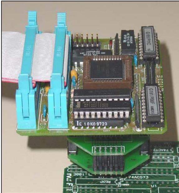
Note that some precaution must be taken to the POD adaptation after the POD is connected to the target. Otherwise, the part soldered to the target may break off.
