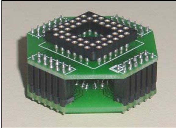
The IA44PGATQ-FIXED represents fixed connection between the POD and the target.
