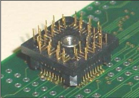
**Phase 2:** Connect the IA44PGATQ-FIXED to the POD. A small adapter is delivered with the POD, converting the default POD target layout to the PGA44 layout. It must be connected to the POD prior connecting the IA44PGATQ-FIXED.
