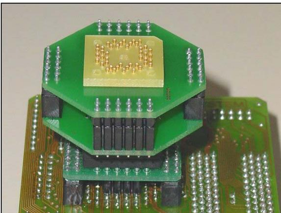
**Phase 3:** Connect the POD to the target via IA44PGATQ-FIXED.
