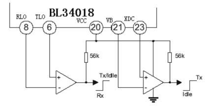
Fig 17 Digital Transmit/Idle/Receive Indication
