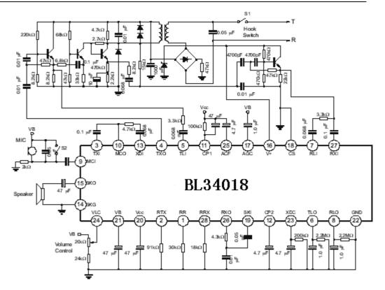
Fig 16 basic Line powered Speakerphone
