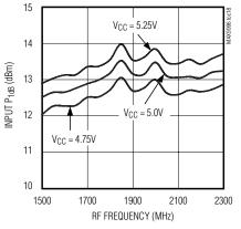
(MAX9996 Typical Application Circuit, V<sub>CC</sub> = +5.0V, P<sub>LO</sub> = 0dBm, P<sub>RF</sub> = -5dBm, f<sub>LO</sub> > f<sub>RF</sub>, f<sub>IF</sub> = 200MHz, unless otherwise noted.)
