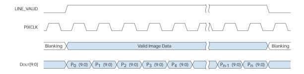
Figure 8: Row Timing and FRAME\_VALID/LINE\_VALID Signals
