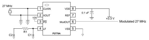
PD selection: Power dissipation can be reduced by completely turning off the IC.
