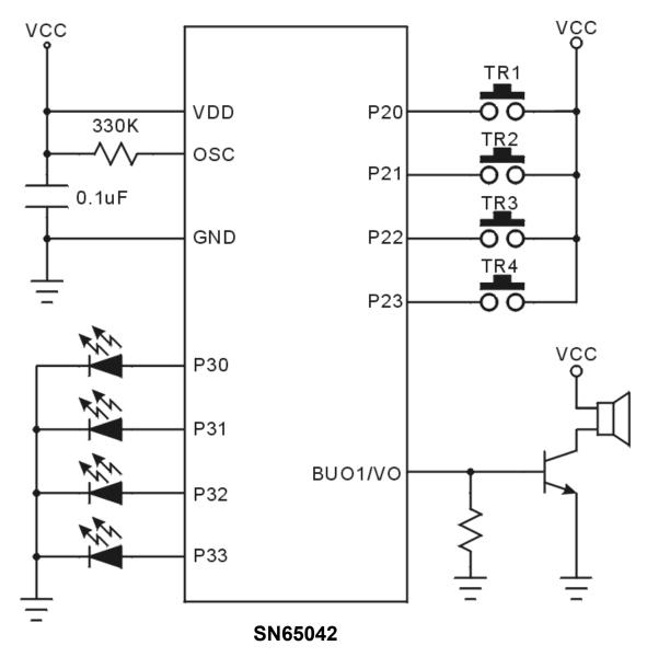
Note: Please bonds all of  $V_{\text{DD}}$  and  $V_{\text{SS}}$  pins.
